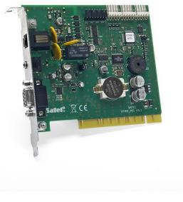
The module supports several transmission formats with automatic recognition and autonegotiation of the communication protocol. The amount of data received by the card is unlimited and their correctness is tested as they come. The card has a FIFO buffer for 250 last received events.
